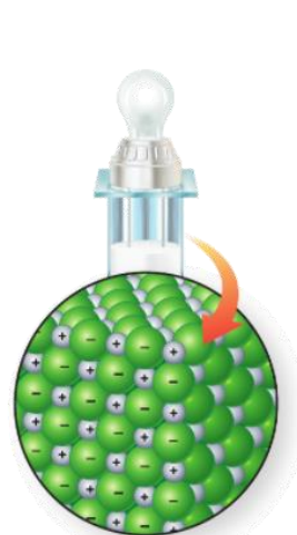
Positive and negative ions fixed in a solid do not conduct a current.
